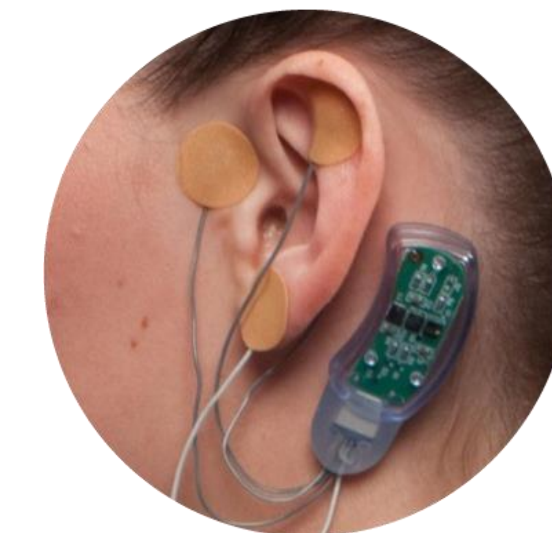
Figure B: The NSS-2 Bridge device placed on the ear. The body of the device is placed behind the ear. The stimulating electrodes are connected via wires and placed at key points on the ear. Each electrode contains a short penetrating needle which is used to provide percutaneous electrical stimulation.
